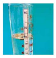
2. Post-production analysis is mandatory if either ethanol or an isopropanol solution is used. Use the alcohol meter to control the alcohol concentration of the final use solution. The accepted limits should be fixed to ± 5% of the target concentration (75%-85% for ethanol).
