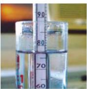
3. The alcohol meter shown in this information pamphlet is for use with ethanol: if used to control an isopropanol solution, a 75% solution will show 77% (± 1%) on the scale at 25°C.
